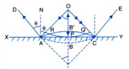
The reflected wavefront AB'C appears to start from I. Hence, I become a virtual image for 0 as a real point object. Draw AN normal to XY, hence parallel to OP.
